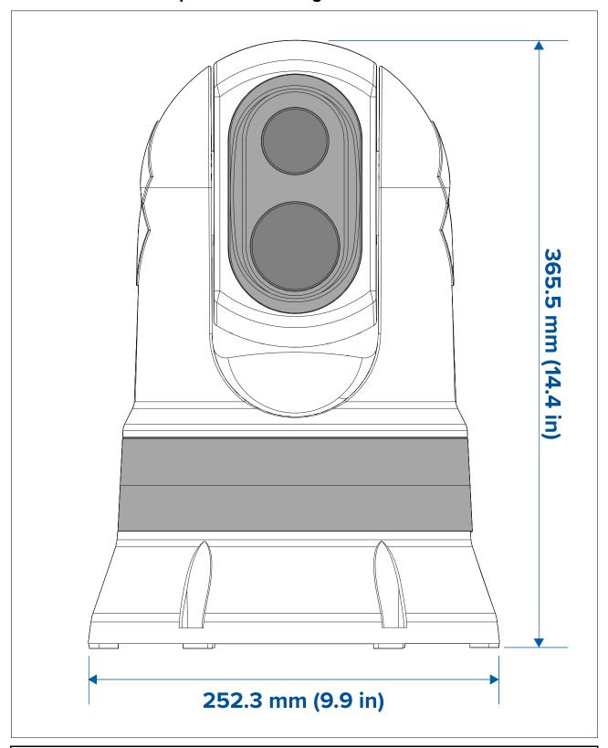
Note: Base diameter with riser base-seal fitted is 254 mm (10 in).
