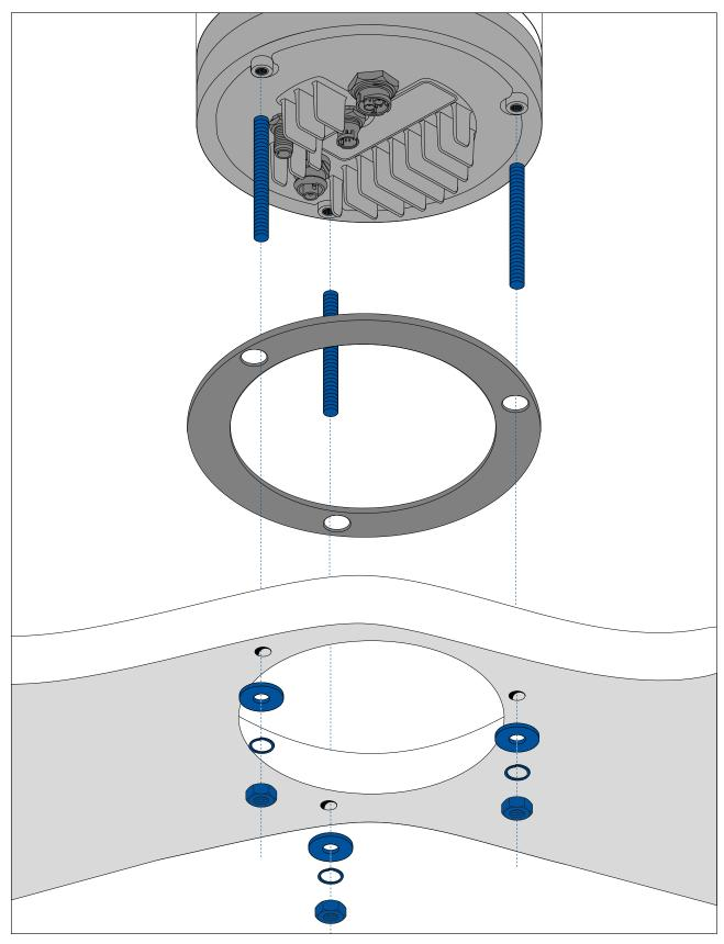
1. Using the template supplied, mark and drill the holes for mounting the camera.
