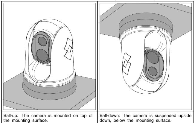
The default video image orientation is for the ball-up configuration; if the camera is to be mounted in the ball-down configuration then the video image must be rotated. To rotate the video image, you must either:
