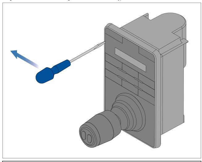
**Note:** To help prevent scratching the product, cover the tip of your screwdriver blade with a small piece of insulation tape.
