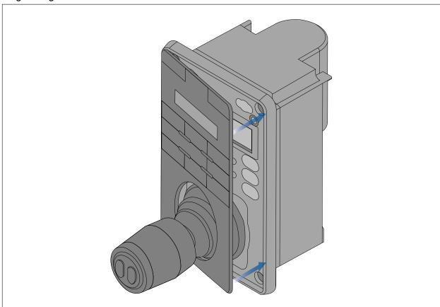
3. Close the opposite end of the keypad mat into the keypad, ensuring that the tab slides into the notch provided. Push all of the tabs on the longer sides into their notches (you should hear a click as each tab engages).
