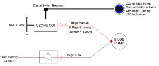
Figure 9. COI Bilge Pump Wiring Example
