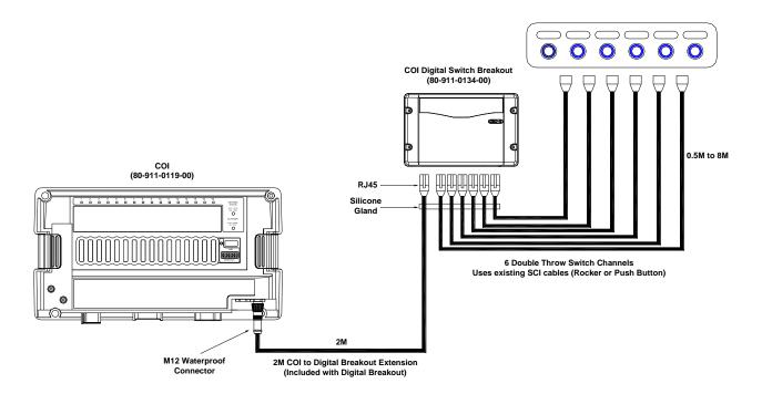
Figure 13. COI Digital Switch Breakout Connections
