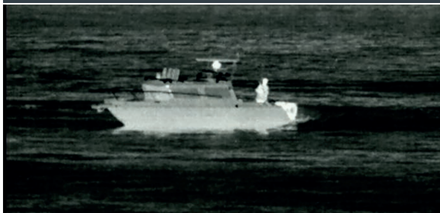
4X OPTICAL ZOOM AND GYRO STABILIZATION ENABLE LONG-RANGE VIEWING OF ONBOARD ACTIVITIES
