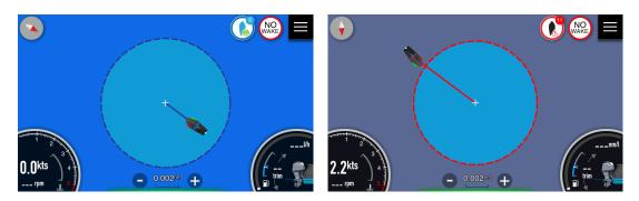
If compass is presented on NMEA2000 network, orientation of vessel is based on compass heading, otherwise vessel is always pointing towards anchor position.
