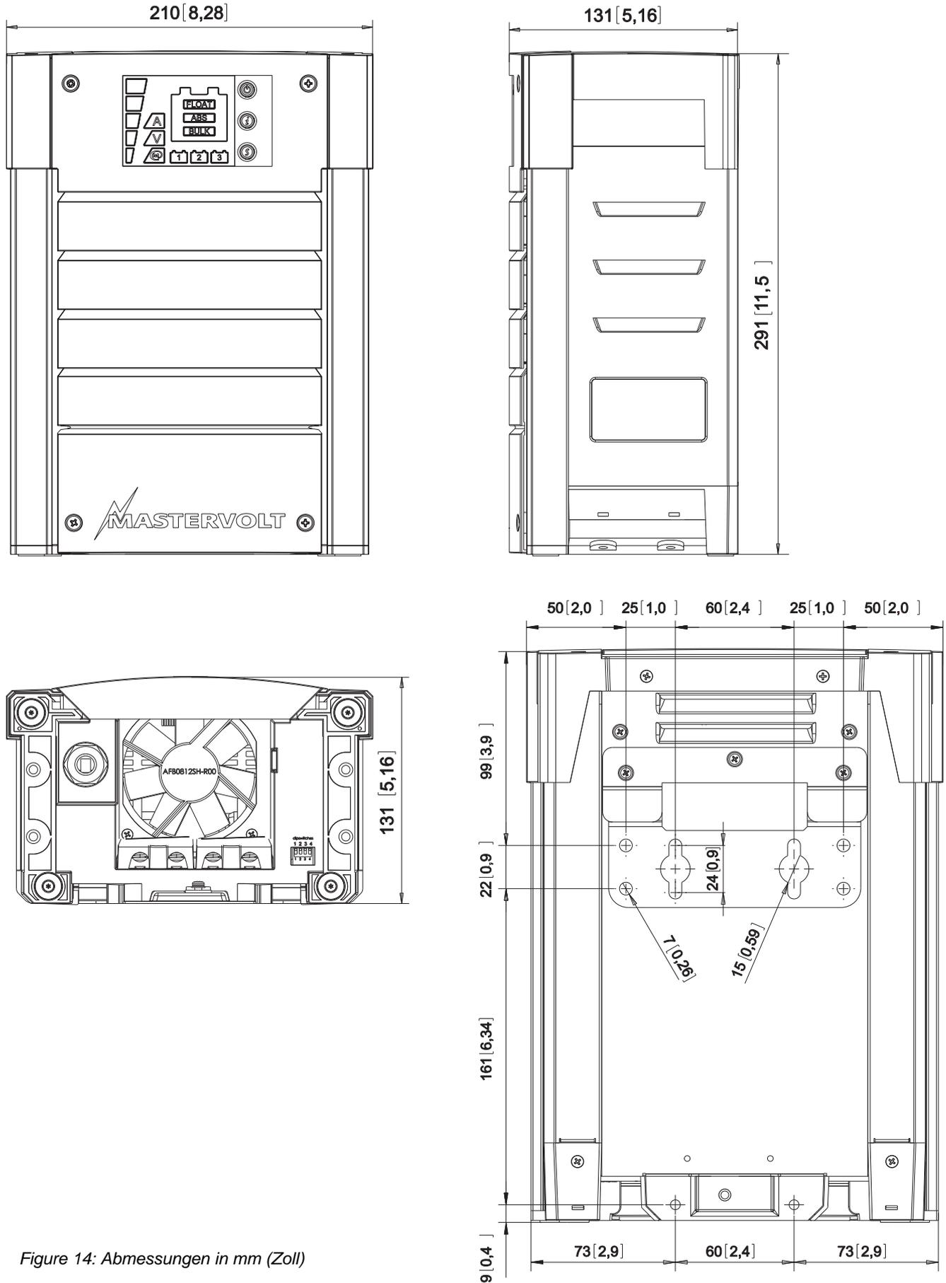
Figure 14: Abmessungen in mm (Zoll)
