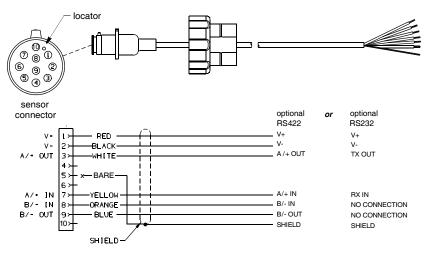
Figure 4. NMEA 0183 sensor cable Copyright © 2007 - 2014 Airmar Technology Corp.
