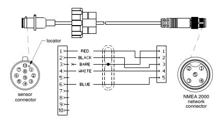
Figure 5. NMEA 2000 sensor cable [6m (20') shown]
