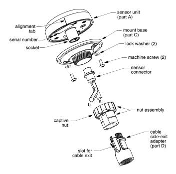
Figure 2. Pole/Rail mount Copyright © 2008 Airmar Technology Corp.
