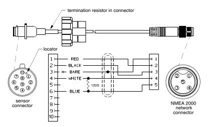
Figure 6. NMEA 2000 sensor cable [10 m (33') shown]
