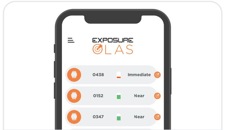
**1.** Ensure a maximum of 6 OLAS transmitters are being tracked. More than 6 OLAS transmitters within range will cause false alarms. If required the addition of the OLAS Core or Guardian allows tracking of up to 15 OLAS transmitters. Disconnect any other Bluetooth devices from your mobile device. Remove and phone cases for testing purposes.
