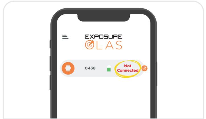
**8.** You may see the tag turn red on the app screen indicating that it has lost signal. If signal is lost for longer than 6 seconds an alarm will sound.
